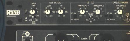
BETTER input section with both mic and line (wireless) inputs that can be summed together
